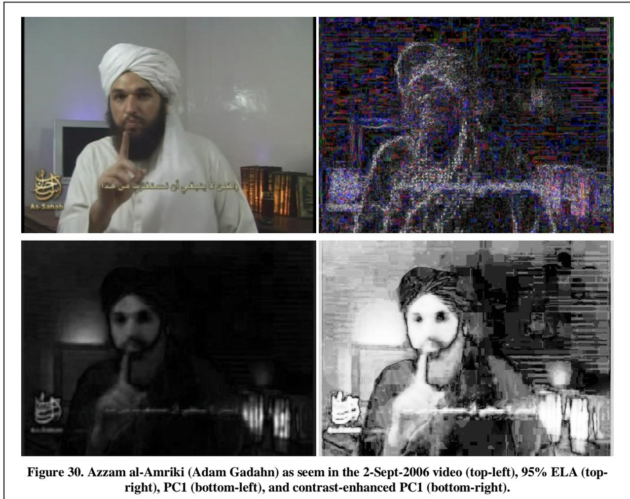
The PC1 with an adjusted contrast shows a horizontal-line pattern. This is a media artifact; the original video of Azzam used an interlaced video source that is identified by the first principal component. However, while the horizontal lines are very visible on the background and mildly visible on Azzam, they are not visible on the books or As-Sahab logo. This suggests that these images did not come from an interlaced video source.
