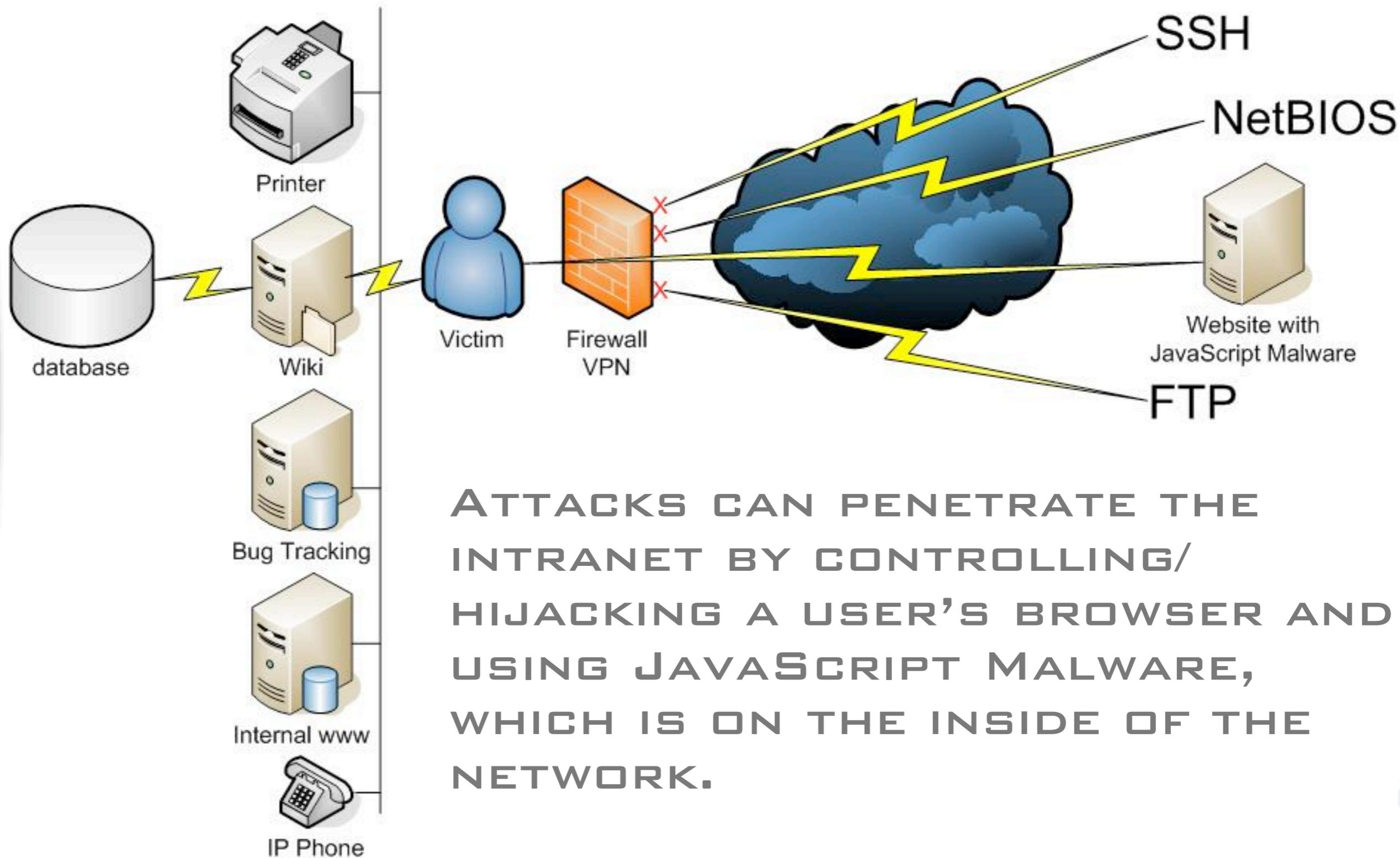
ATTACKS CAN PENETRATE THE INTRANET BY CONTROLLING/ HIJACKING A USER'S BROWSER AND USING JAVASCRIPT MALWARE, WHICH IS ON THE INSIDE OF THE NETWORK.
