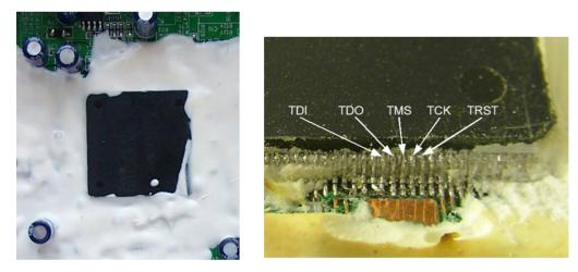
• Glue can be removed with chemicals or hot air
