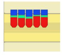
Mastering of locks (the issuance of multiple levels of permission) is achieved by the insertion of an additional pin (often called a "wafer" because of how thin it is) into the stacks. This allows for multiple levels of clearance at the shear line... and while that makes for more functionality, it also can make the lock easier to pick.
