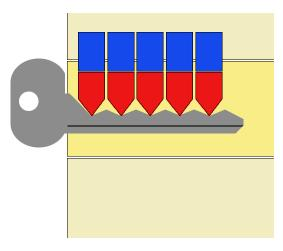
The bump key attack involves the insertion of a specially-cut key into the lock. If the head of this key is struck with appropriate force, the ridges of the key will all simultaneously smack against the bottom pins and the energy of this strike will cause the top pins to all jump upward. The resulting gap leaves the shear line without any binding force. If the plug is turned at the exact right moment, often the lock will open.
