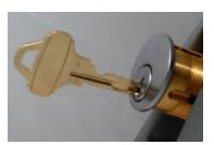
The Everest key has a long groove down the side. This channel catches and then raises the check pin. While this is an interesting and rather nice system, there is no variation in the size, position, and functionality of the check pin. It is the same size and operates the exact same way in all Schlage Everest locks.
