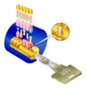
prevents the impressioning attack described above in the traditional dimple lock section.
