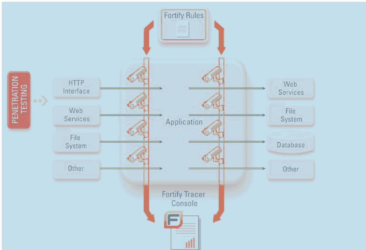
Here, we have monitors looking at both incoming & outgoing traffic through the application, as well as the execution of security critical functions. The monitors are controlled through a centralized 'rules' file for modularity, and the results of what the monitor sees is fed into a 'console'.
