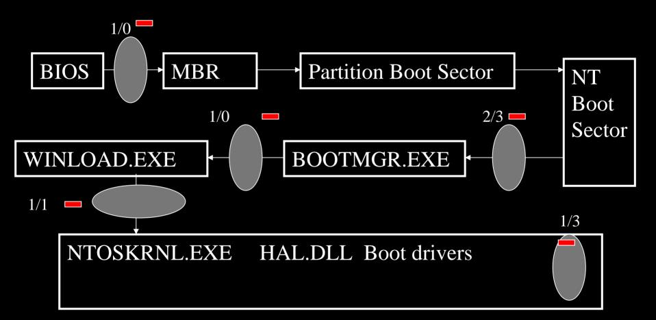
NOTE:- The ovals shows the point where Vboot kit hijacks control. The first number shows detours applied to next stage and second number shows patches applied. A red block shows relocation
