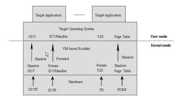
There is no concepts of Host OS or Guest OS in this new VMBR scheme, thus no need for a Total Context Switch that is absolutely necessary in Type II VMM, the OS being controlled by VMBR is referred to as Target OS.
