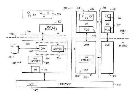
Diagram 1—3 The Whole Structure of VMware Workstation
