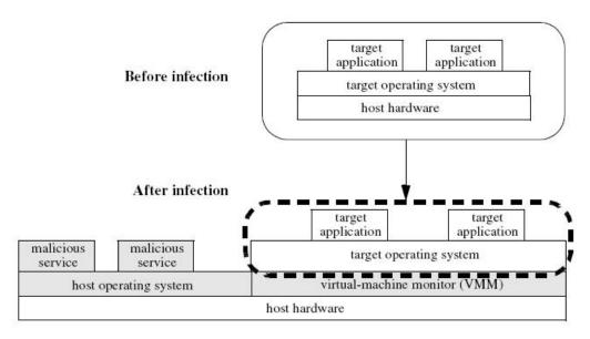
Diagram 2-1 The Working Principle of SubVirt
