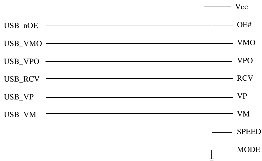
Figure 4-2. Single-Ended USB connection
