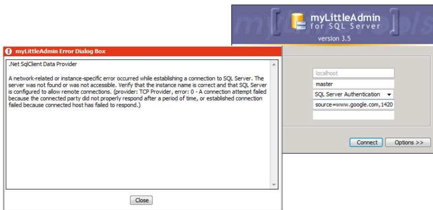
Fig. 6. A connection cannot be established through the XX port to www.google.com
