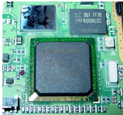
Figure 3: Glue around the edges of BGA packages on Sprint PCS phone
