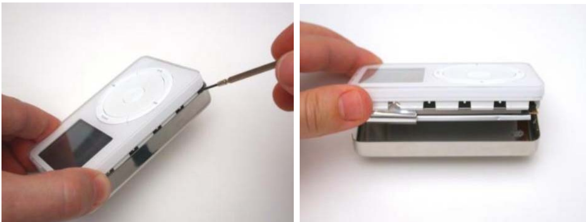
Figure 1. Opening the housing of an Apple iPod using a jeweler's screwdriver, from Grand, et al.'s Hardware Hacking: Have Fun While Voiding Your Warranty [14]
