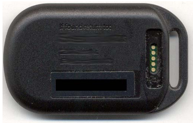
Figure 2. External interfaces on a hardware authentication device
