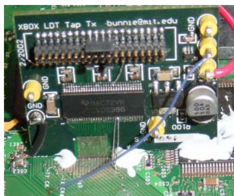
Figure 5: Huang's Xbox HyperTransport Bus tap circuit, from http://www.xenatera.com/bunnie/proj/anatak/xboxmod.html
