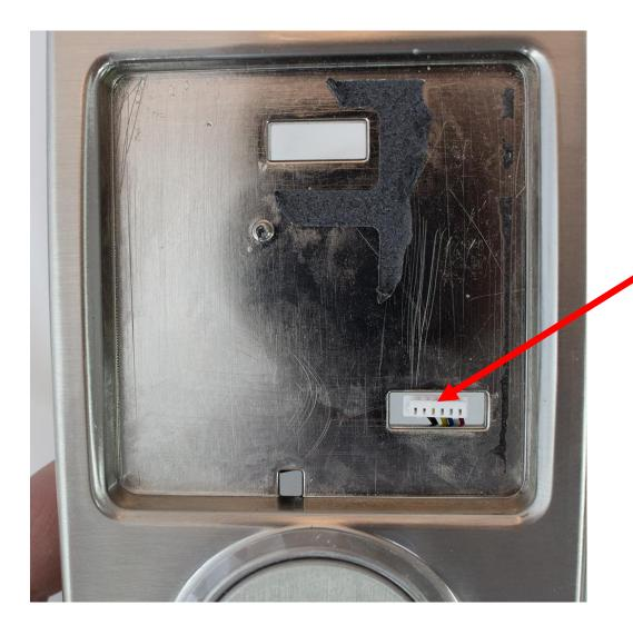
+VBAT (From 4x AA Cells) +3.3V (for logic) Serial RX/TX
