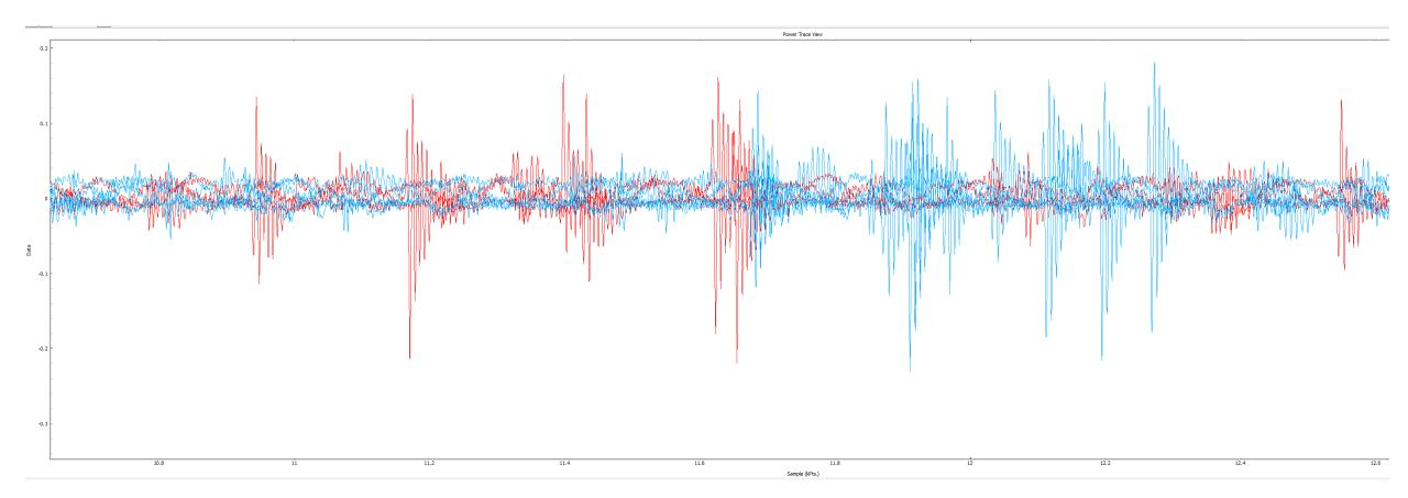
Appears power spikes measurable at front keypad... Also opens up power analysis. Following slides show preliminary stages of this work (measuring at backend instead):
