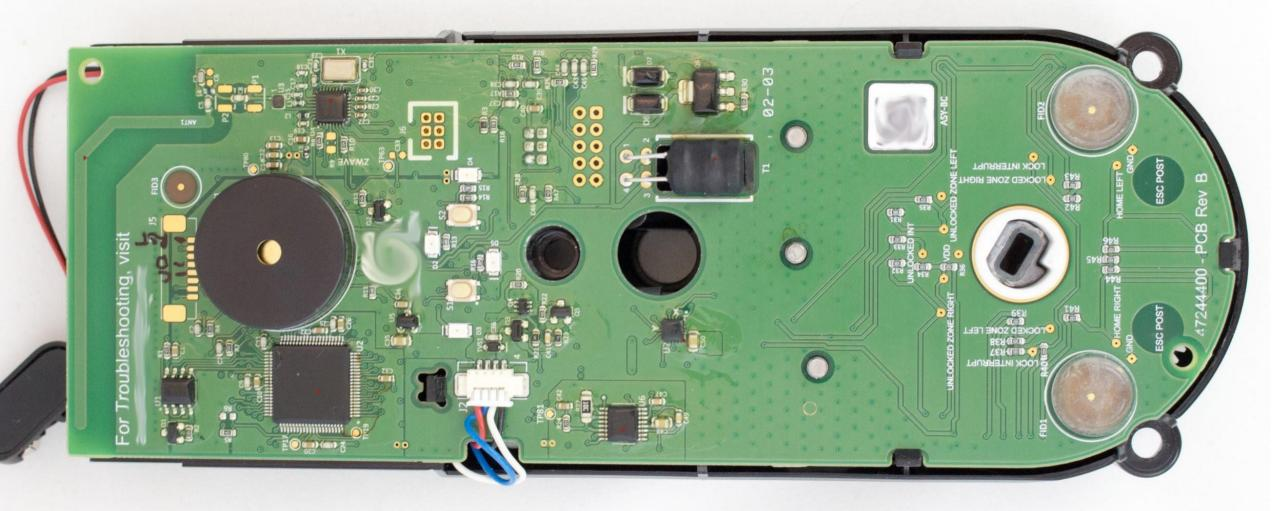
PIC18F87K22 Microcontroller DRV8833 – Motor Driver LIS3DH (Or similar) – Accelerometer
