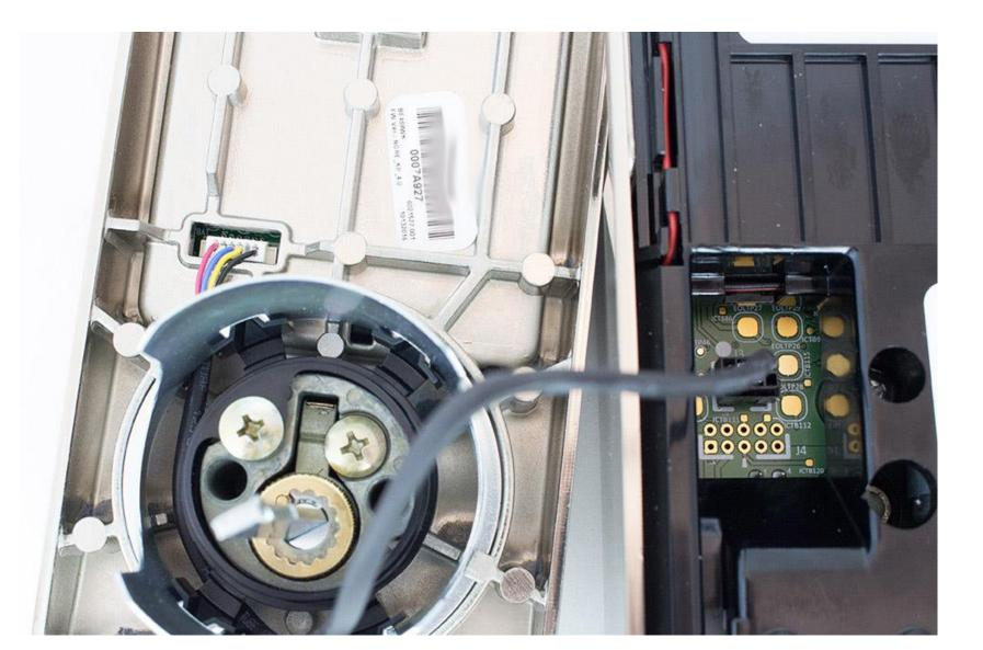
PCB Antenna ZW0301 – Zwave Radio + Microcontroller (SoC) Transformer to make very loud siren
