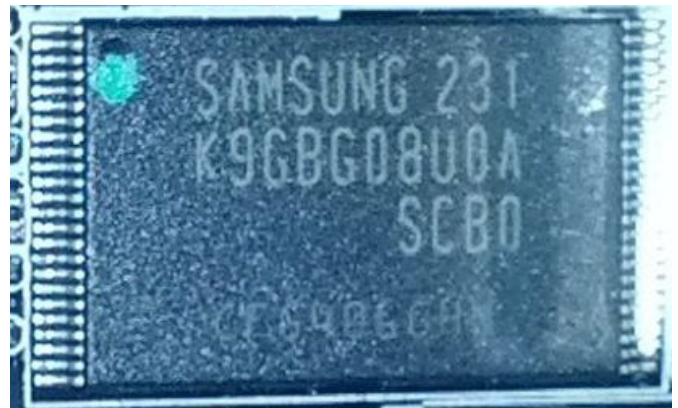
Figure 3: NAND Flash in Thin Small Outline Package
