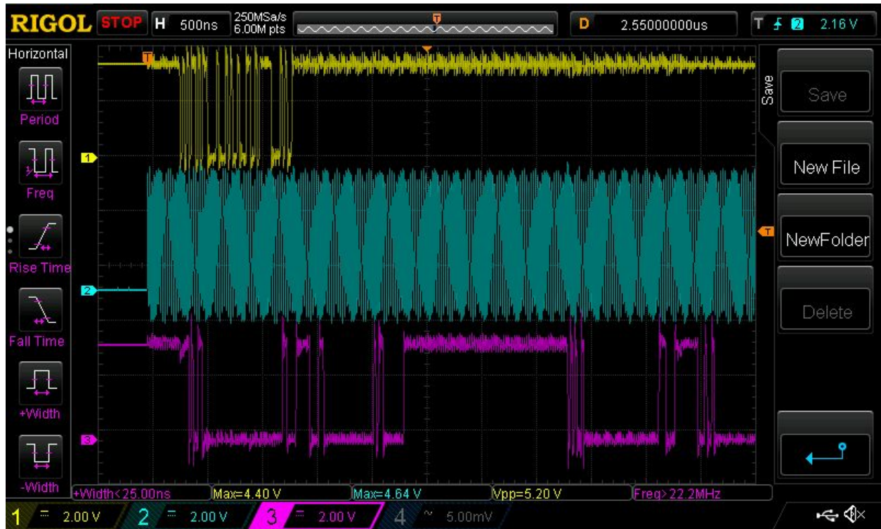
Figure 13 - Scope capture of CMD signal
