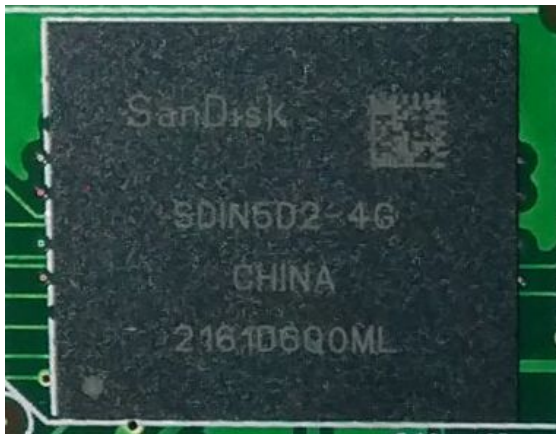
Figure 2: eMMC Flash in Ball Grid Array Package
