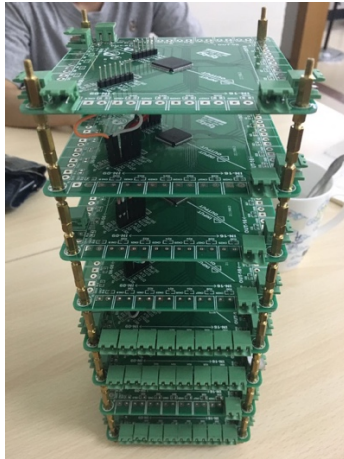
Figure 2: Eight AD75019 are cascaded to implement a 128 x 128 array
