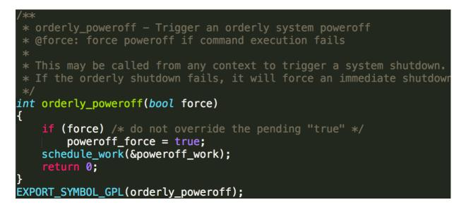
orderly\_poweroff() will create a worker thread to create a new user mode process "/sbin/poweroff". The path of this executable file is poweroff\_cmd which can be manipulated.
