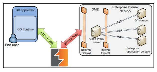
Figure 16 – Normal traffic flow using a proxy
