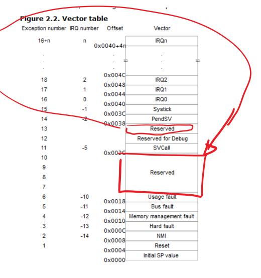
On system reset, the vector table is fixed at address 0x00000000.
