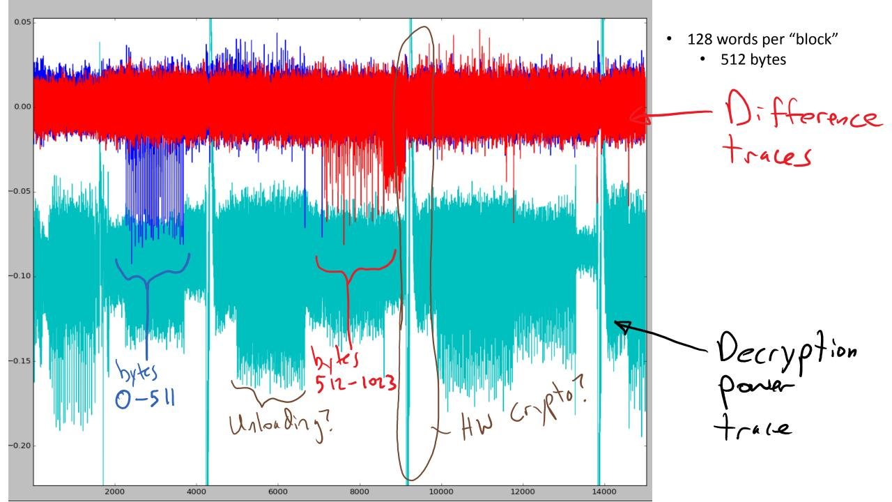
FIRMWARE ATTACKS 1) Can cause arbitrary code to be decrypted. 2) Can move interrupt/reset vectors quazi-blindly. 3) If could determine either (a) part of stream cipher or (b) part of code (init routines?) may be able to build short "dum nor" "dun per"
