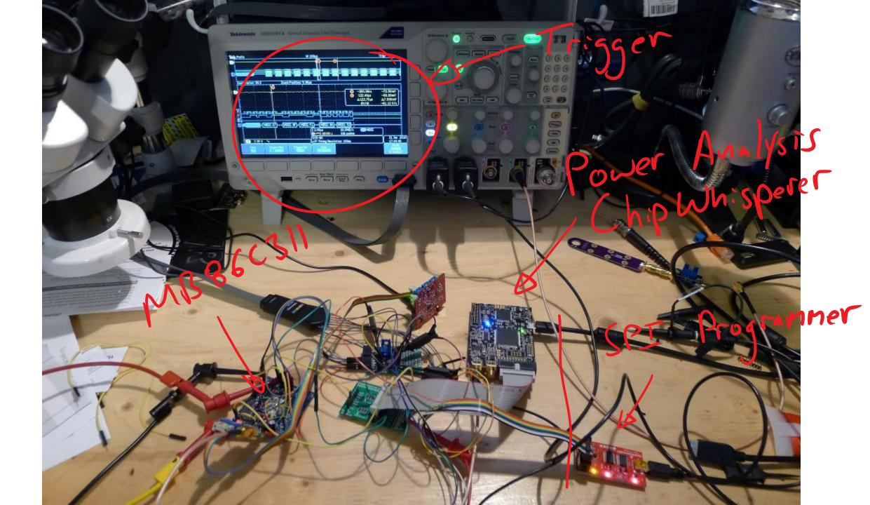
DOWER ANALYSIS 1. Program SPI Flash with pattern. 2. Reset MB86711, will reload FLASH. 3. Capture power at different places
