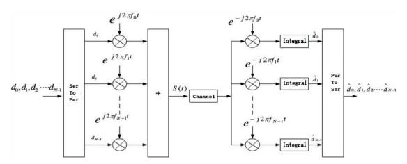
The symbol rate is T, the bit rate is Ts, because the relationship of serial to parallel transform, so T=NTs.
