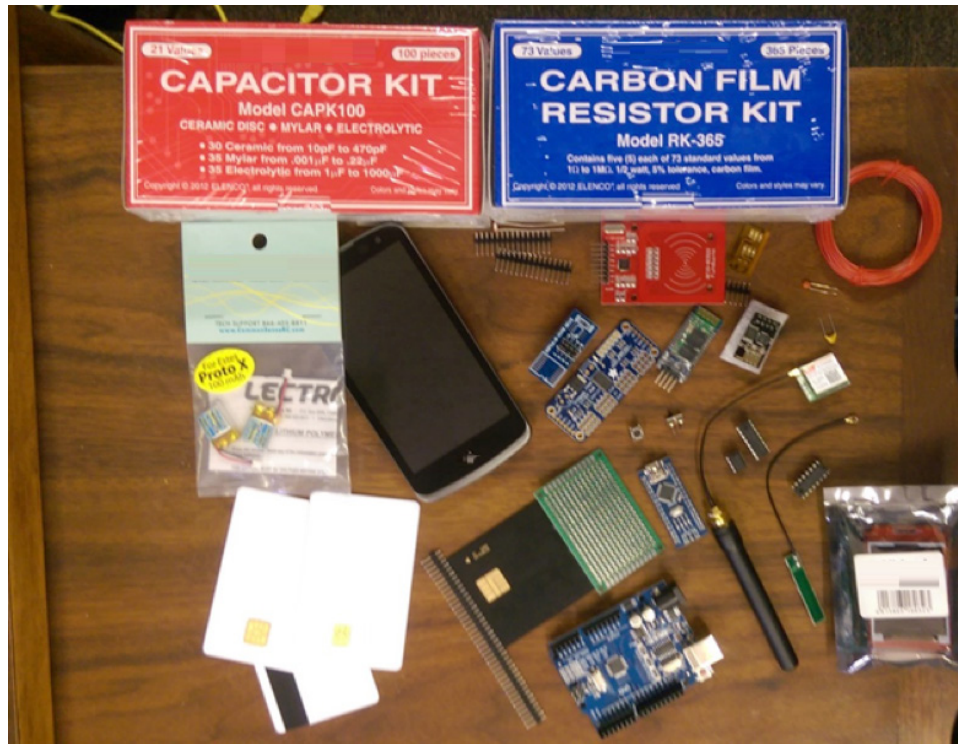
Figure 5: Setup needed to relay the three most common transaction types: EMV, NFC, and magstripe.
