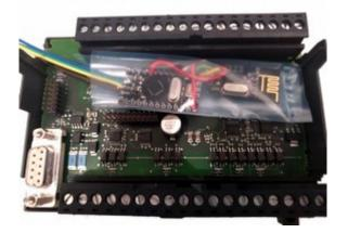
Using sample code available directly from Arduino, the implant listens for a command to set an output to high when it receives a '1', low when it receives a '0' and high-impedance when it receives an 'x'.
