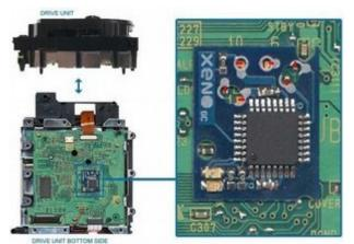
tampering with a couple wires, these modchips are able to undermine the hardware and software security of game consoles to enable home-brew, cross-region, backed up, and pirated games. While the hardware aspect which often means installation requires soldering to a relatively expensive piece of consumer electronics — limits adoption of hardware modchips, it is often the hardware mod chips that enable further research and understanding of systems that eventually make soft-mods possible.
