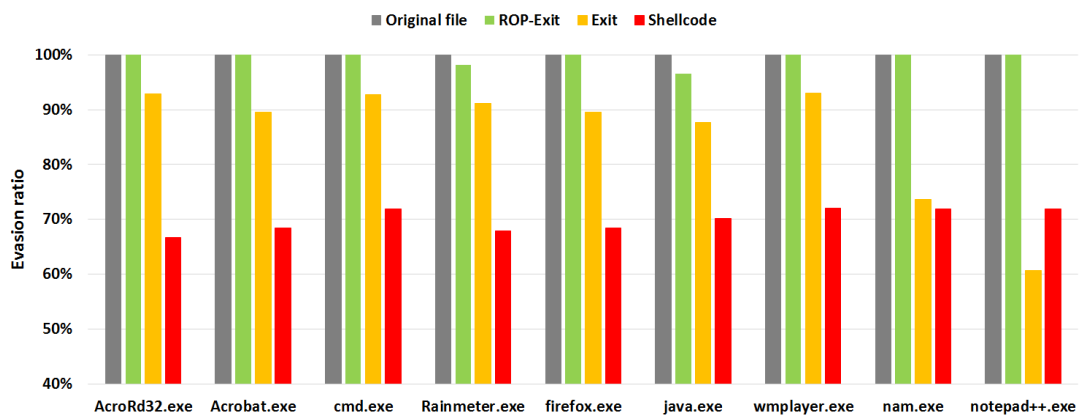
Figure 3: Evasion ratio of ROPinjector for the reverse shell payload
