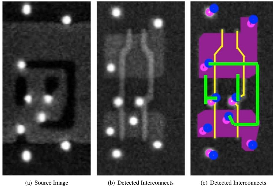
Figure 3: SEM images of the polysilicon and metal 1 layer of a NOR gate, see Figures 3(a) and 3(b). Through a semi-automated process, the entire cell library of a device can be reconstructed with ARES. The resulting representation of the gate within the database of ARES is also presented, see Figure 3(c).
