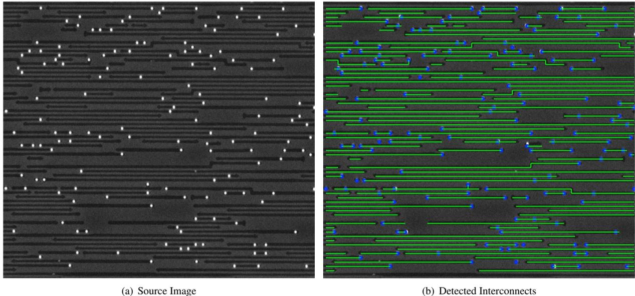
Figure 2: SEM image of the Metal 3 layer that has been corrected for distortion, see Figure 2(a). The features detected by the ARES analysis suite are visible in the image with the extracted features, see Figure 2(b).
