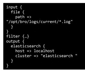
Figure 2: Logstash Permanent Configuration
