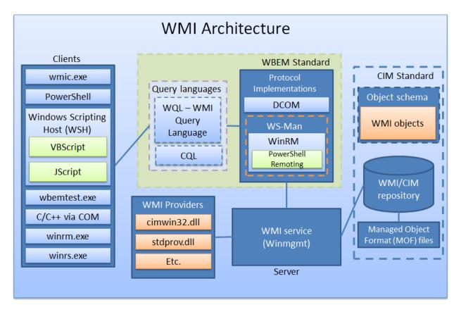
Figure 1: A high-level overview of the WMI architecture
