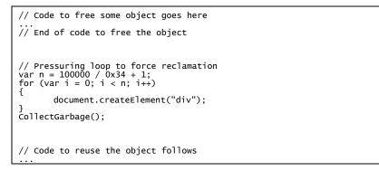
Figure 2 Pressuring code example
