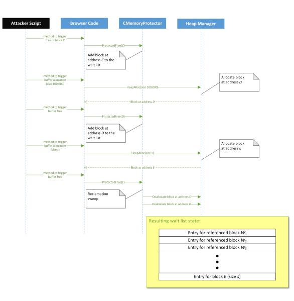
Figure 6 Diagram of strategy for clean deallocation of a block at address C
