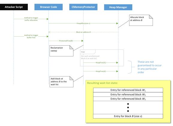
Figure 5 Sequence diagram for reclamation sweep and block add to wait list
