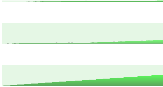
Figure 4. Heap state evolution for tcmalloc . The axes are as in figure 3. As can be seen, the layout resulting from the same series of allocations is drastically different between the two allocators. In figure 3 the allocations are grouped together with most successive allocations simply being placed at the next highest free address. In contrast, tcmalloc results in these allocations being spread out over a much larger area of memory (resulting in the 'zoomed out' viewpoint). 2
