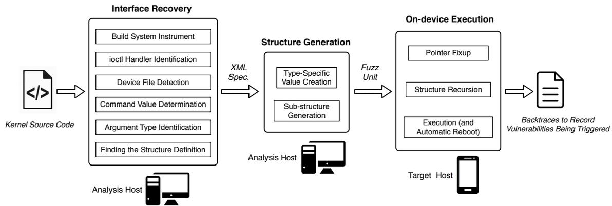
**Figure 1: The DIFUZE approach diagram.** DIFUZE analyzes the provided kernel sources using a composition of analyses to extract driver interface information, such as valid ioctl commands and argument structure types. It synthesizes instances of these structures and dispatches them to the target device, which triggers ioctl execution with the given inputs and, eventually, finds crashes in the device drivers.
