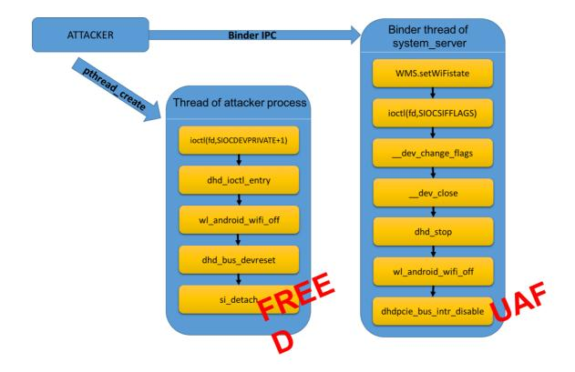
To trigger the UAF, the binder thread has to enter *wl\_android\_wifi\_off* soon after attacker's thread enter it. The window is small. If the re-filled object meet following requirements, it will reach a macro INTR\_OFF, *intrsoff\_fn* is a function pointer can be controlled by attacker.
