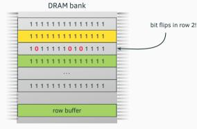
• Capacitors leak  $\rightarrow$  refresh necessary
