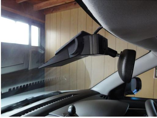
Figure 2: MobilEye C2-270 installed (on the windshield) with the display at the bottom.
