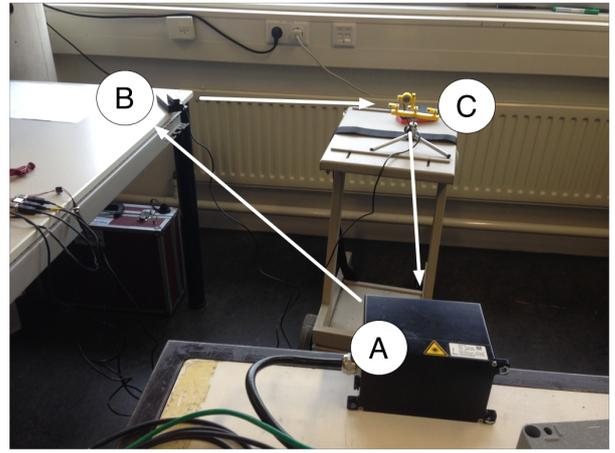
Figure 6: Setup of a LiDAR relay attack
