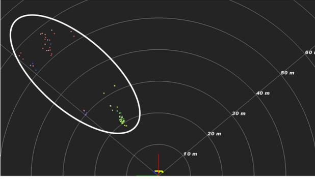
Figure 7: Result of LiDAR relay attack. Light pulses are received from the left, and relayed from the right.
