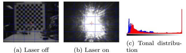
Figure 4: Blinding MobilEye C2-270 with 650 nm laser
