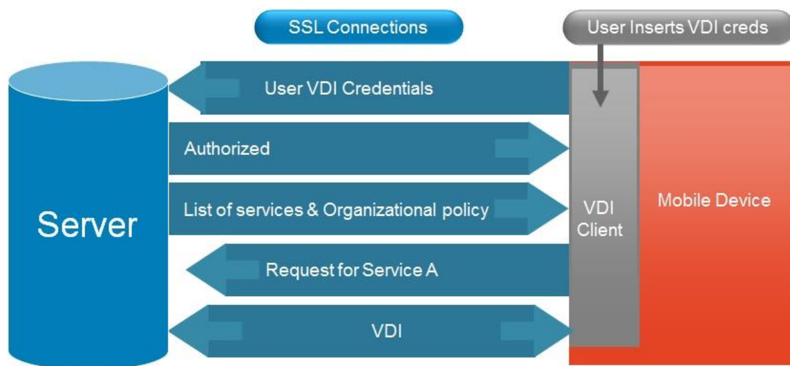
Overview of VDI server-client communication
