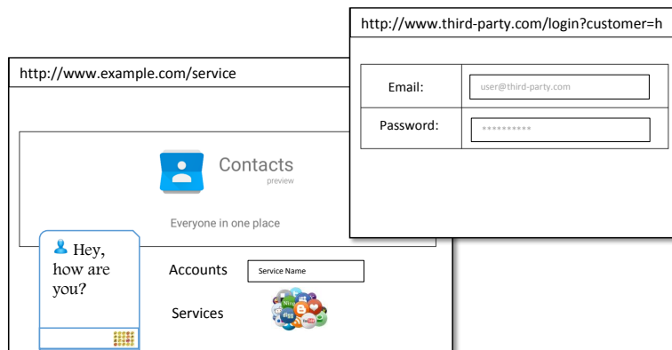
Figure 2.2: Requesting third-party resource access without losing the content of the currently open document.
