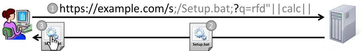
Figure 1 – The three steps attack flow of reflected file download
