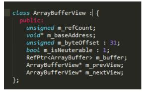
Changing ArrayBufferView::m\_buffer pointer can achieve Arbitrary Address Read/Write (AAR/AAW). And the size of ArrayBufferView is 0x40.
