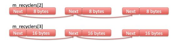
In the past, UAFs in RenderArena can be easily exploited. Overwriting the "Next" pointer to a controlled buffer which is outside the Arena, the new allocation of objects of that size may return that controller buffer to the program. The exploiter can then leak the important pointer out to bypass ASLR and manipulate the RenderObject to get IP control.
