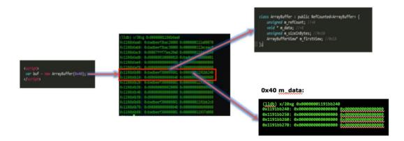
When ArrayBufferView is assigned, WTF::ArrayBuffer.m\_firstView will point to an ArrayBufferView structure:
