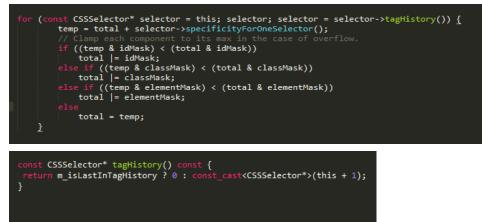
So we have to put another fake CSSSelector structure right after and set m\_isLastInTagHistory (the 18<sup>th</sup> bit of the bit value) to 1 to quit the loop ASAP and avoid the code keeping OOB read which will finally crash.
