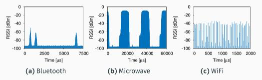
Figure 2: Noise in wireless channels (Boano et al. 2012)
