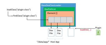
Figure 3: Hook ClassLoader to Launch Plugin without Installation
