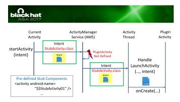
Figure 6: Replace the Intent content with Stub Activity Class
