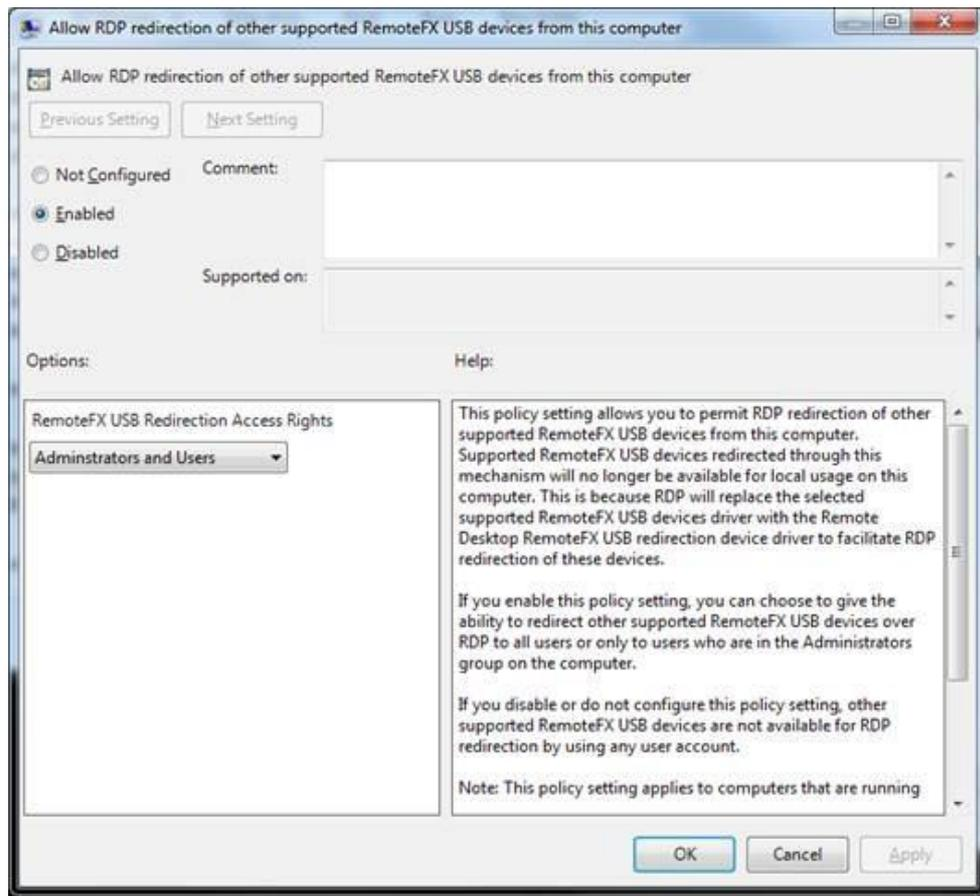
Figure 5: Local Windows policy setting to enable RemoteFX USB redirection
