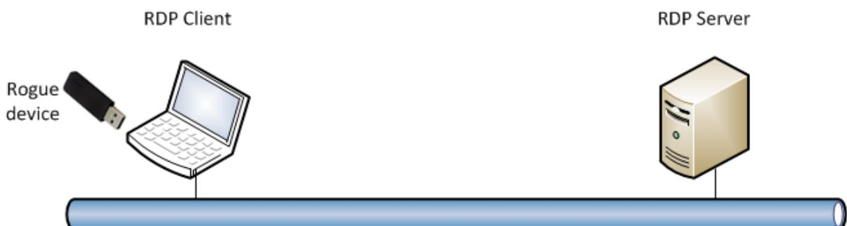
Figure 3: A rogue USB device is connected to the client
