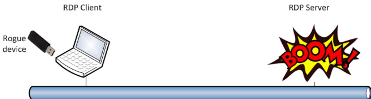
Figure 12: The rogue device is now inserted and will be redirected via RemoteFX USB redirection
