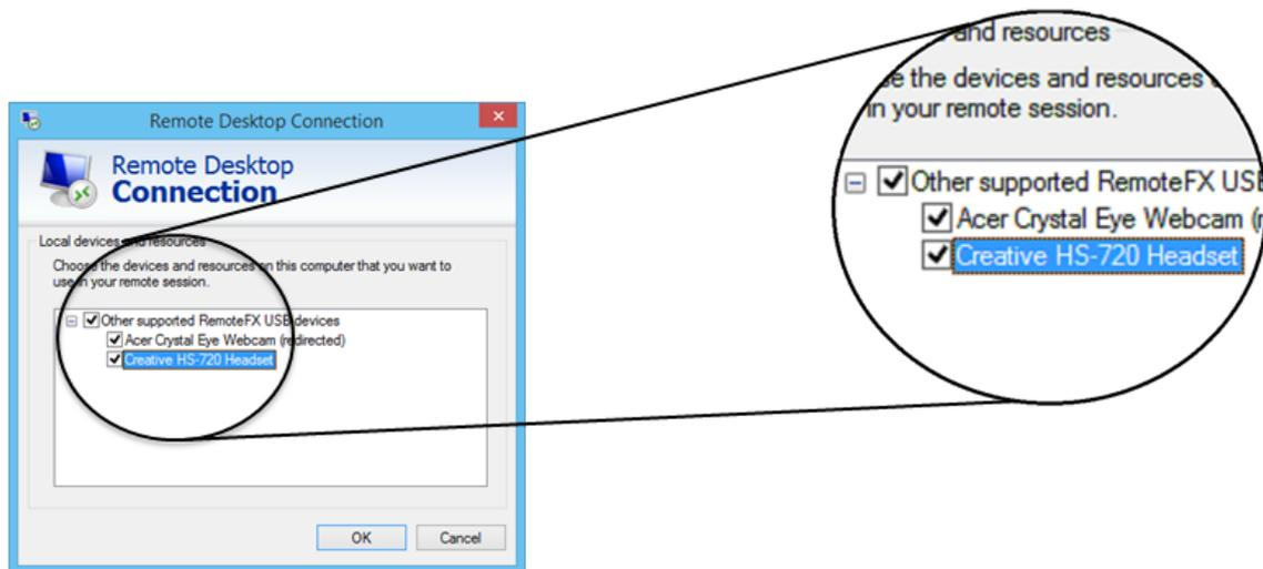
Figure 11: The USB devices that can be redirected via RemoteFX USB redirection
