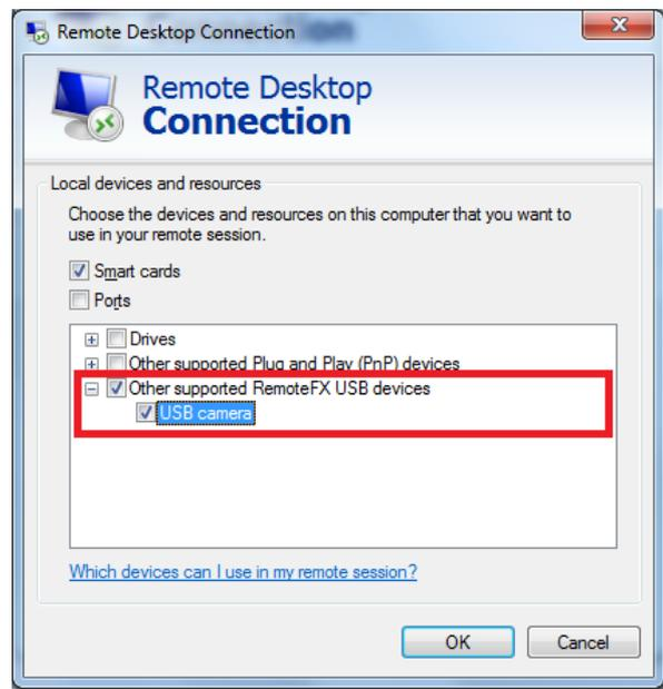
Figure 7: RDP client RemoteFX USB device settings
