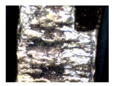
At 1,500 uses (roughly 1.5-2 years of use) a distinct change in the appears of the pins. The key has been used so many times that the milling marks have almost completely been removed. Again, slight scratches on the pin are being caused by the key becoming more jagged as it too wears down.
