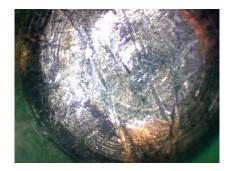
The act of using a pick tool is invasive, and we expect the stronger material of the pick tool to cause marks on the softer brass or nickel-silver of the lock components. In the photo (left), we see scratches where the pick tool was used to lift the pin. These appear to be single-pin picking marks due to their shape, size, and position.
