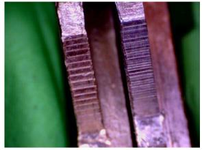
When a key is duplicated with a stylus-based key machine a mark is left on the side of the original key (left). This is due to the stylus being gently dragged against the key, and resembles a long, straight, polished line. This cannot be confused with wear of the key because it is not in the direct center of the key.
