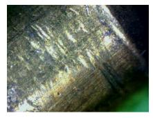
Because we are forcibly binding bottom pins at or above the shear line we expect to see marks on the pins where this occurred. In the photo (left) we can see several marks where the pin was bound against the plug in the form of straight lines sheared into the pin. (Note: the scratches to the left are pick marks)
