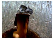
The face of a lock that has seen moderate to heavy use will have many dents and imperfections caused by normal use. How many times have you went to unlock a door and slightly missed the keyway? In the photo (left), many small dents and scratches from normal use are visible.
