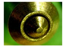
The marks left by an attacker are in many ways indicative of their skill level. In this photo (left), deep and plentiful pick marks are shown. The attacker, an amateur, used extreme force on both tension and pick tools. The extreme tension causes pins to bind against plug and require more force to be lifted.
