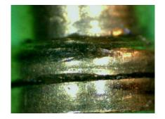
The act of key bumping basically slams the key against the bottom pins to allow for kinetic energy to be transferred from the key to the top pins. Because they are immobile and absorb the kinetic energy, this causes considerable damage to the bottom pins in the form of large dents. In the photo (left), a large dent is visible on the pin, inconsistent with normal wear (and lockpicking or pick guns, for that matter).
