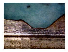
Keys can be duplicated in many ways, but the most common is duplication by hand or with a key machine. Identifying an original vs. duplicate key is an important function of the forensic locksmith. In addition, the forensic locksmith may be able to determine if the key was recently duplicated. Which of these two photos shows the original key, and which is the duplicate. Why?
