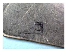
Cam manipulation is one of the most common bypass methods. The American 700 (old models) suffer from this vulnerability. Essentially, the cylinder is not required to move in order to actuate the cam. In the photo (left), tool marks left on the cam and back plate indicate that bypass was used as the method of entry.
