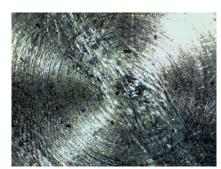
Tensions tools used in lockpicking also leave identifiable forensic evidence. When we take the plug apart, we can usually find light scratching and scuffing at the front of the keyway. Marks can be at the top or the bottom of the plug, depending on the tension preferences of the attacker, and how clear they are may help us determine their skill level. In the photo (left), light scratching and a definitive tension tool mark (the line) are visible.
