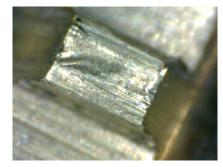
Inside the plug we also expect to find various forensic evidence. In this photo (left), the plug walls have scratches are various angles that are inconsistent with the use of a key.
