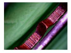
Possession of keys that are made by hand are, in a general sense, somewhat suspicious. In most cases hand made keys are easily identified by measuring the ramp angles, shoulder to first cut distance, and the distance between cuts. Hand-made keys generally have imperfect, jagged ramp angles and poorly spaced cuts.
