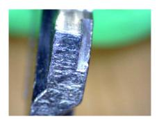
New pins are clean, with no dust, grease, or dirt. Light abrasions and corrosion may exist depending on how the pins were stored prior to being used in the lock. Factory original pins usually do not exhibit these characteristics. A clear indication that pin has not been used is the fresh milling marks around the tip of the pin.
