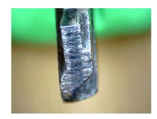
After 250 uses (roughly 3-6 months of use) a ring develops around the pin. This is the key gliding under the pins, spread around the tip because insertion and removal lightly rotates them back and forth. The key is also lightly polishing the pins, too.
