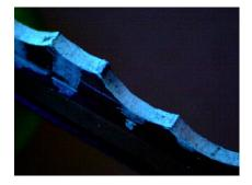
Various materials are transferred to the key during use. Generally hair, fiber, and fingerprints will be examined by a crime lab. The forensic locksmith, however, may examine the findings of the crime lab to identify the uses of materials found on keys. In this photo (left) we see a light green residue, which happens to be modeling clay.
