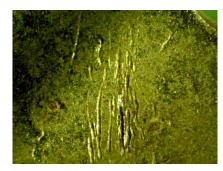
The striking of the pick gun needle against the bottom pins causes very clear forensic evidence. Unlike picking, which causes scratches, the pick gun causes impact marks that, when done many times, begin to resemble the spokes of a bicycle along the circumference of the pin. In this photo (left), several impact marks are visible.
