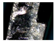
At 5,000 uses (roughly 5-6 years of use) the front pin (left) has no milling marks, and almost all scratches have been polished away. From this point on wear looks similar to this, with light markings sometimes being created by wear of the key.
