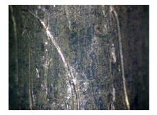
For the attacker, it is difficult to not touch the sides of pins. This can happen during raking as well as single-pin picking. Marks left on the sides of pins are quite noticeable and not as prone to wear and those in the center of the pin. In the photo (left), light scratches at varied angles are visible.
