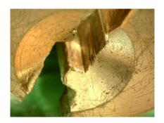
The pin chambers within the plug may also be damaged by bumping. When kinetic energy does not properly transfer to the top pin, the pin stack may instead press against the chamber walls (caused by the movement of the bump key). Repeated bumping may cause these areas to distort, stretching in various directions. In the photo (left), the pin chamber is stressed is distorted in many directions, but mostly to the top left.
